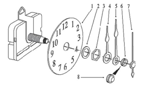
1 Place clock body so that the shaft is going through the hole on the front of the clock and the base is hiding on the back side.
